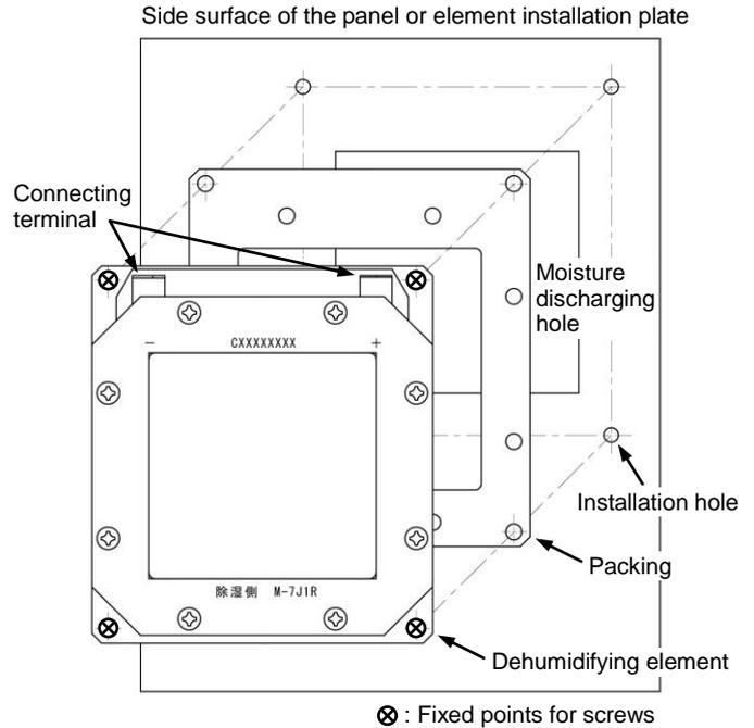
Fig.2 Installation method
