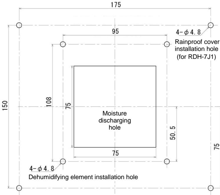
Fig.1 Installation dimensions
