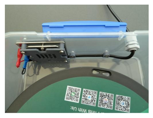
M-2J1R size 2 membrane mounted in a small filament drying enclosure
