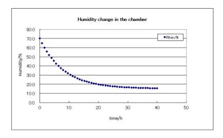
Drying simulation for a 125-litre enclosure in a 70% RH 18°C ambient using a size 3J membrane and leakage area of less than 3.4 cm<sup>2</sup>
